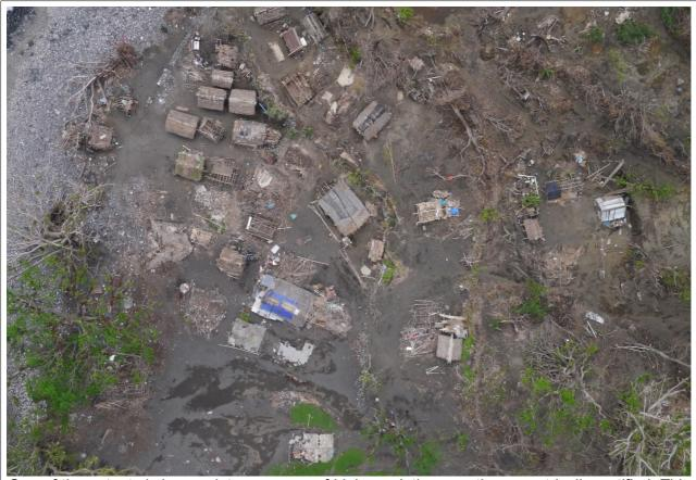
One of the outputs is image data coverage of high resolution exactly geometrically rectified. This can be superimposed over the satellite image data.
