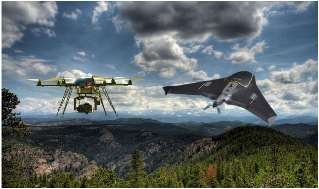
Now, both UAVs are working in synergy. The SPC fixed wing covers larger areas within short time. The copter UAV has the potential to fly slow which support high image resolution and is capable to look onto the objects from different view angles and fly around larger infrastructure elements. These options allow the creation of three dimensional datasets without shadow effect. The fixed wing and the copter UAV produced image data and DEMs can be merged to seamless datasets.
